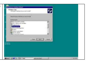
From Manufacturers list, choose ACTISYS, from Infrared Device list, choose ACTISYS IR-200L Serial Infrared Device for IR200L; click Next>.
